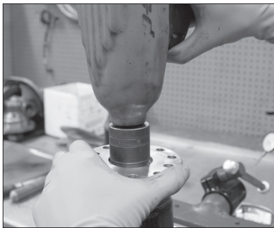
1/2" impact gun on pinion nut setting.
