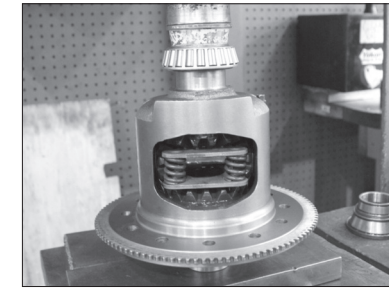
Pressing on carrier bearing
